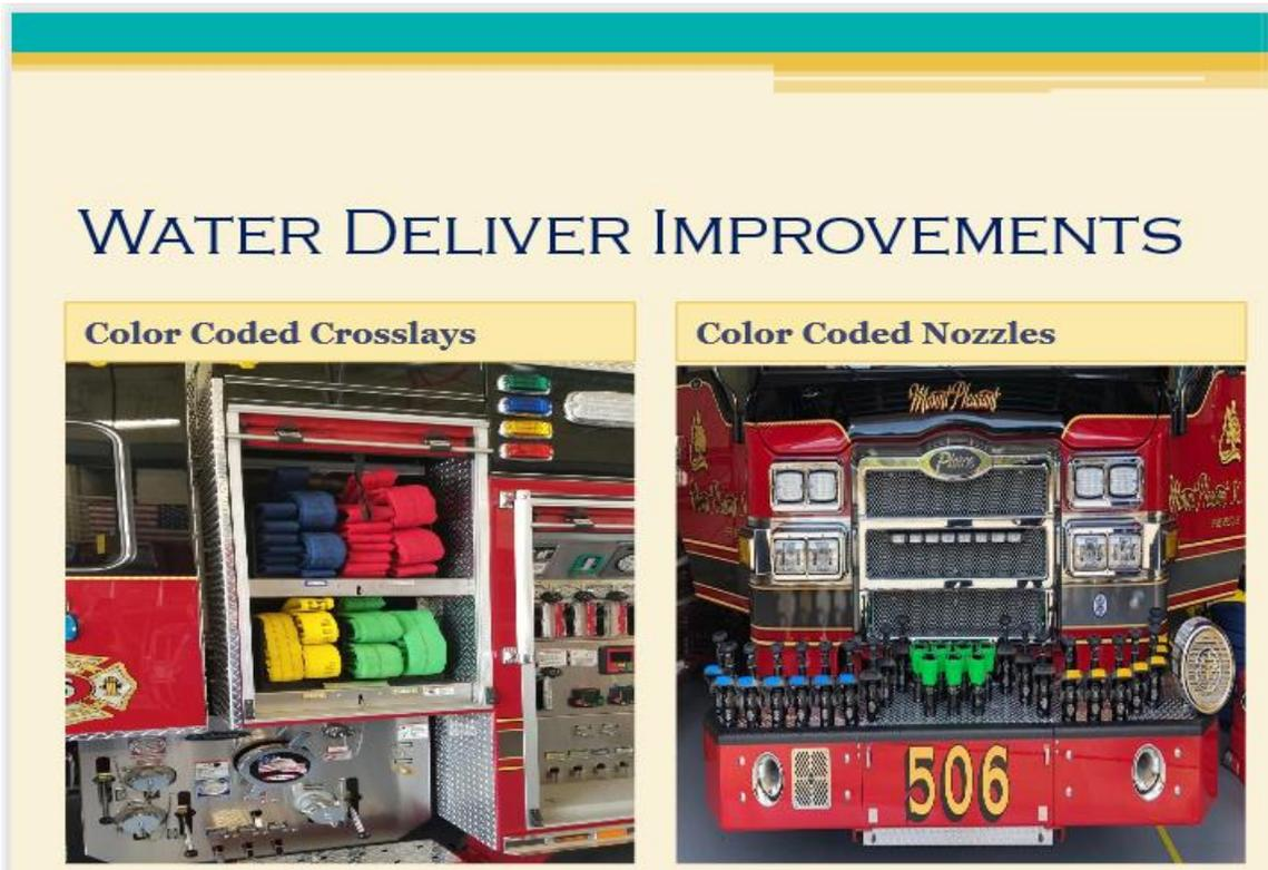
He said color coding the nozzle to the hose helps ensure that more water is delivered to the fire.
